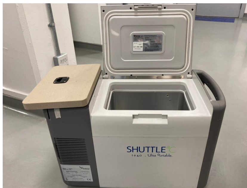
Figure 2.7: A portable freezer capable of transporting samples at temperatures as low as -80°C. Image by Fiona Allan.
